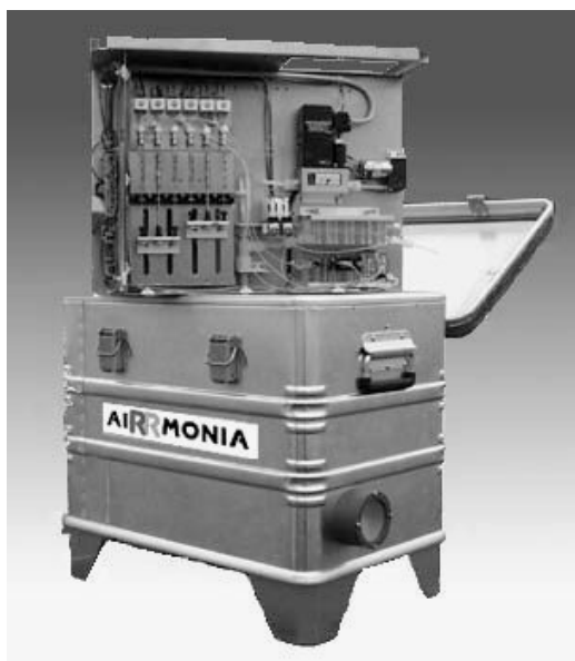
Figure 1.2 Image of the aiRRmonia monitor for ambient ammonia. 17
